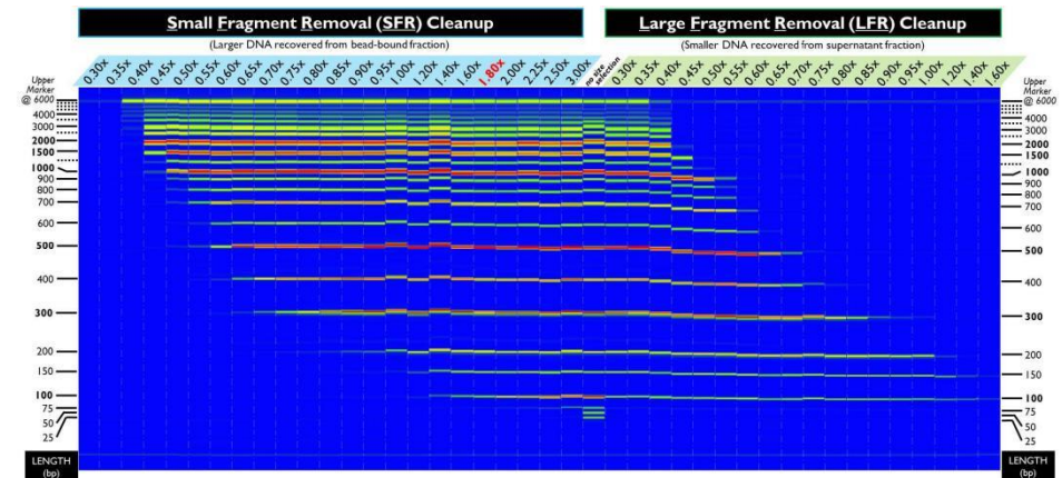
Fig.1 Pseudogel image from the fragment analysis of DNA recovered after size selection.
